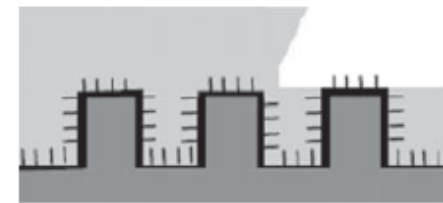
Wenzel filled microstructure
