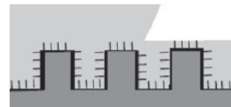
Wenzel filled micro/nanostructure
