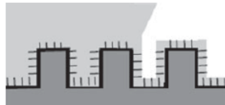
Wenzel filled nanostructure
