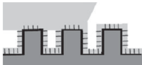
Cassie filled nanostructure
